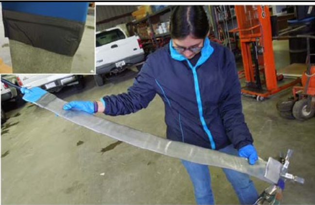
Figure 7. GSI Environmental Engineer Luz Rocha with the section of wick drain. Inset: Duck-bill connector attached to the top of the wick drain.
